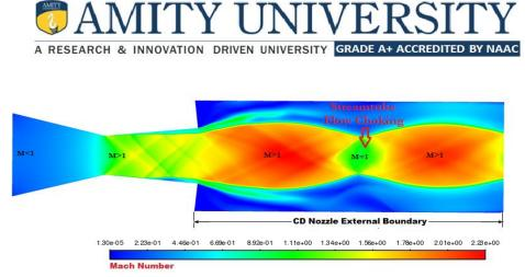
Fig. 2 In silico demonstration of sonic-fluid-throat effect in an external flow.
