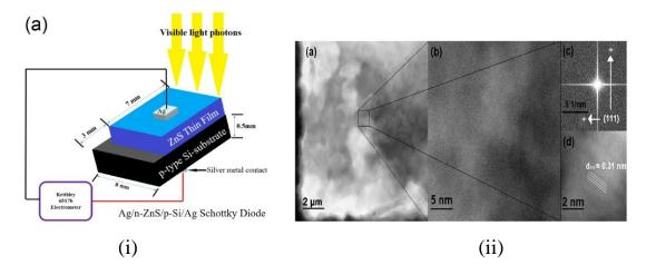
(a) Schematic illustration of the fabricated Ag/ZnS/p-Si/Ag
