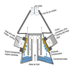
Figure 1: Schematic diagram of proposed atmospheric water generator
